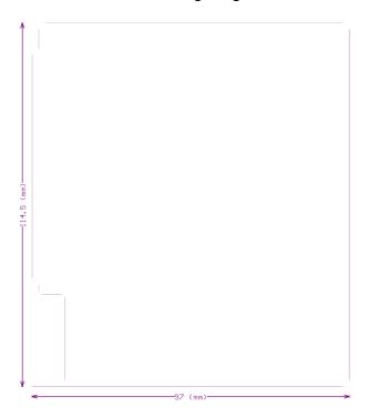
PCB size drawing (PCB size 97\*114.5\*1.6mm)
